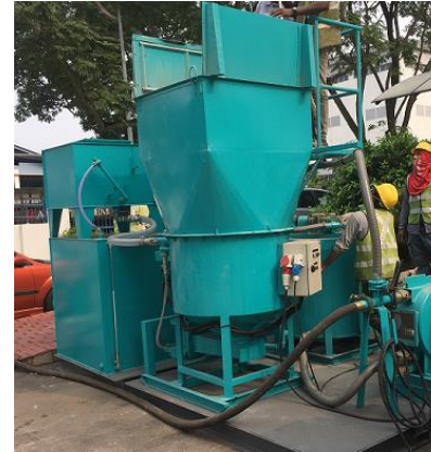
(a) Mixing With Big Mixer (500kg powder/batch)
