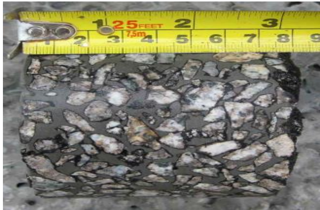
W/P: 0.25, Fluidity: 27 sec, thickness: 80mm
