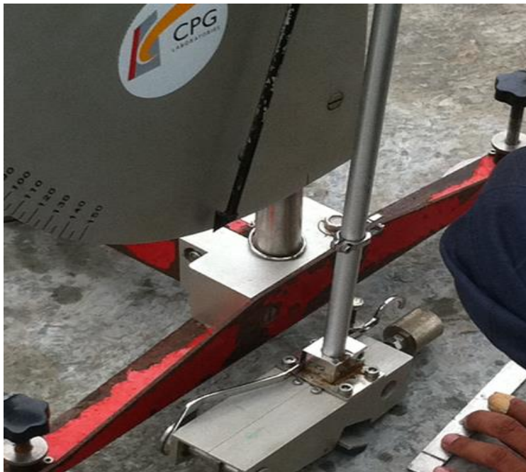
Skid Resistance Measurement by ASTM E303
