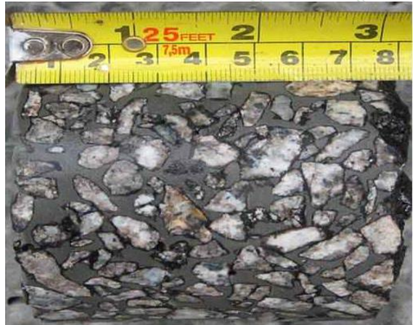
(b) Cored Sample (75mm thick)
