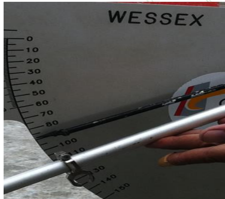
Skid Resistance Measurement by ASTM E303
