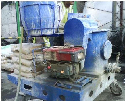
(b) Mixing With Medium Mixer (100kg powder/batch)
