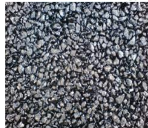
(f) Compacted PAC Surface (Air Void 25-30%)
