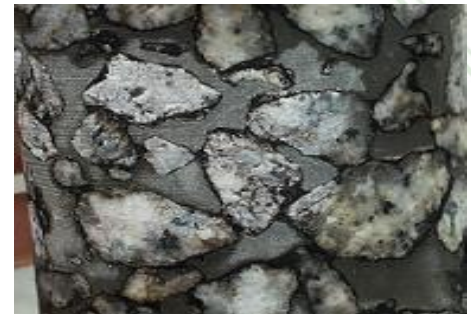
(c) Semi-Rigid Pavement (Cored Sample)
